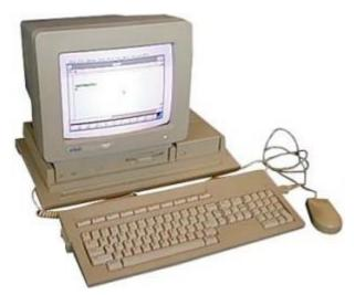
The Atari Mega STE was Atari Corporation's last ST series personal computer, released in 1991. The MEGA STE was essentially a latemodel 680×0-based STE mounted in the case of the otherwise unrelated Atari TT computer, although a number of TT features were also blended in. The resulting machine was a more business-like version of the ST line.
